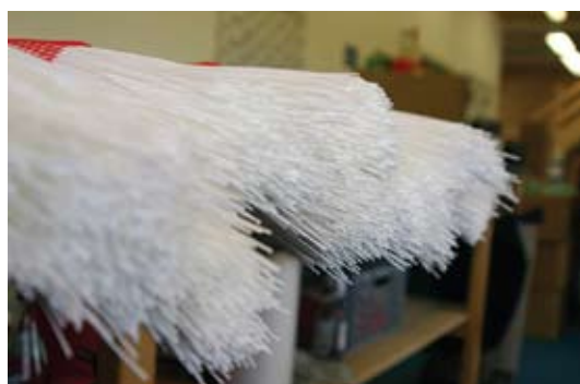
Figure 2. Membrane fiber bundles before being processed into elements.
